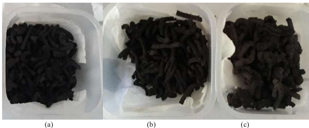
Figure 1. Combined biopellet fertilizer of biochar: chicken manure: fish waste a) 70:15:15; b) 50:25:25; and c) 20:40:40.
